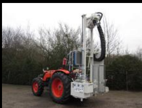
Tractor Drill Rig
